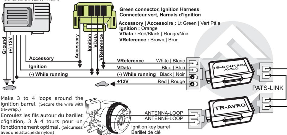
Make 3 to 4 loops around the ignition barrel. (Secure the wire with tie-wrap.)
