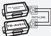
Connect the **TB-AVEO** module to the **TB-CONTROL AVEO** using the PATS-LINK cable.
