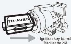
Place the **TB-AVEO** module close to the front of the ignition barrel.
